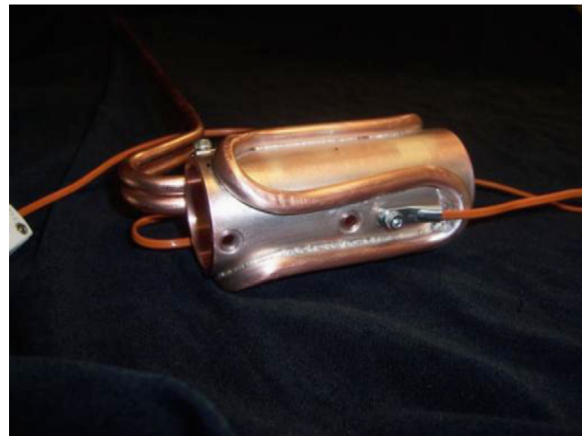
Fig. 5. Picture of the cryogenically cooled 3(1/2) in long, 1(1/4) in inner diameter (1/8 in thick) copper cylinder. The attached copper refrigerant tubing and optical access holes are shown. The interior is coated with graphene material Aquadag.
